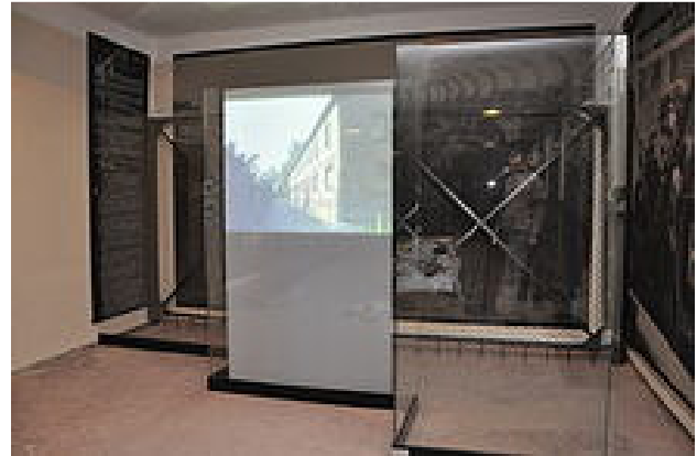
Polyvision Smart Glass, projection mode
